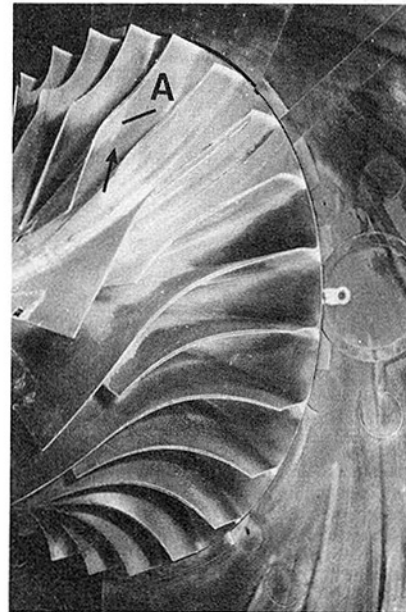
Fig. 9 Colored dye pattern deposited on the pressure surface showing a line A separating the leakage flow region near shroud from the trailing edge zone as the origin of reverse flow
